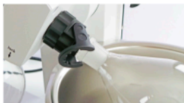
EASY CLIP open, Flask unsecured
